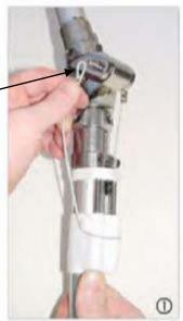
Swing Phase with Extension Assist: Adjust the spring tension by turning the screw with a 4mm hex wrench on the adjustment ring.
